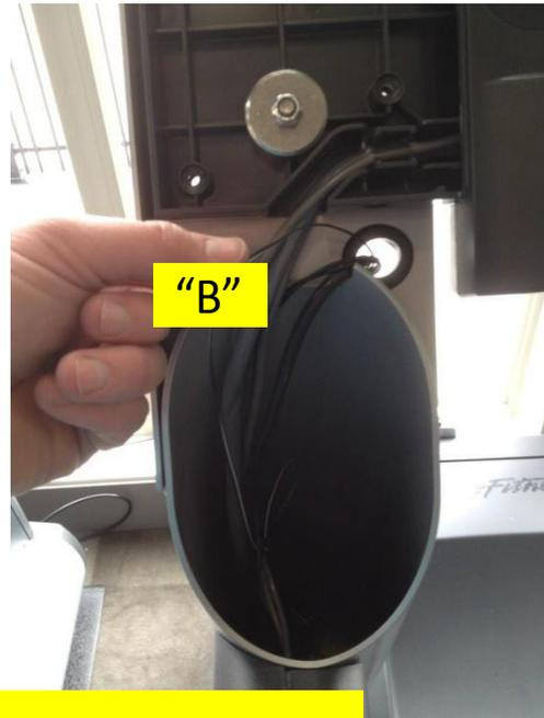
3. Pull through AUXIR cable taped to pull tape and reinstall cap, secure CAB at screen, and adhere emitter on face of cable/satellite box
