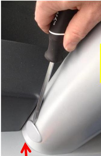
1. Remove cap at base of Treadmill leg
