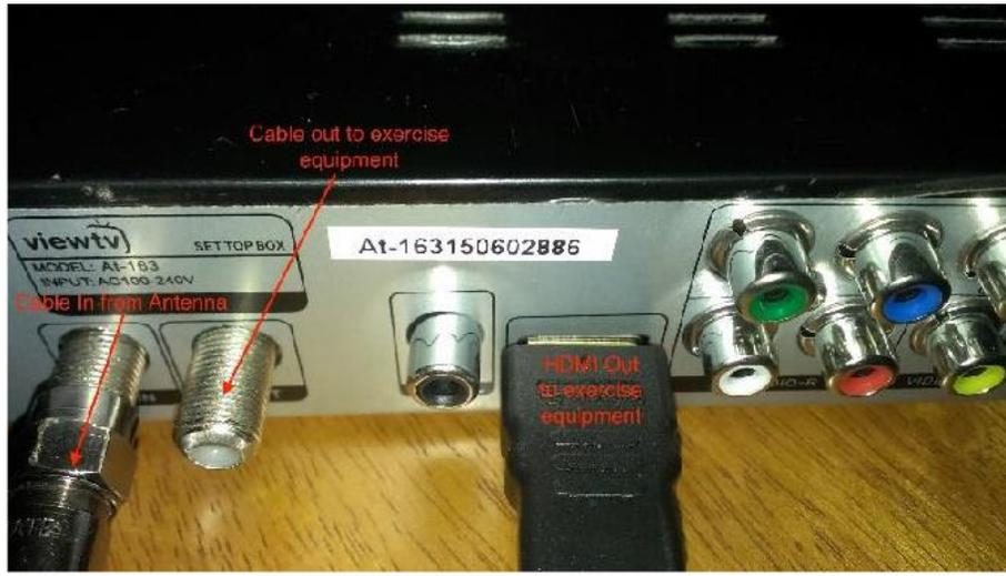
2. Connect the other end of the cable to the HDMI or Coax ports at the base of the machine.
