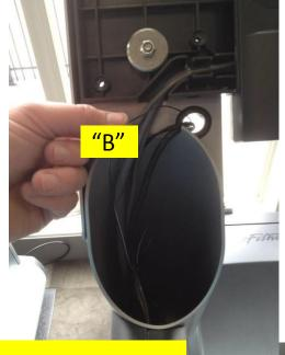
3. Pull through AUXIR cable taped to pull tape and reinstall cap, secure CAB at screen, and adhere emitter on face of cable/satellite box
