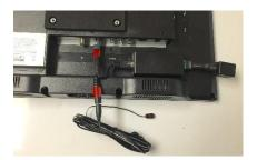
6. Once the CAB is hooked up you will need to run the IR emitter cable down the machine to the base of the cardio. There it will connect to either the set top box or a cat5/6 cable for sending the signal to an AV closet.
