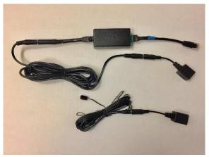
5. After the IR cable has been run through the machine the IR emitter should be placed over the infrared eye on the front of the set top box. If you cannot see where the IR eye is on the front of the STB, shining a flashlight at the front of the box will usually help you to see the IR eye. Please see the IR eye locations of some of the most common STB's below:
